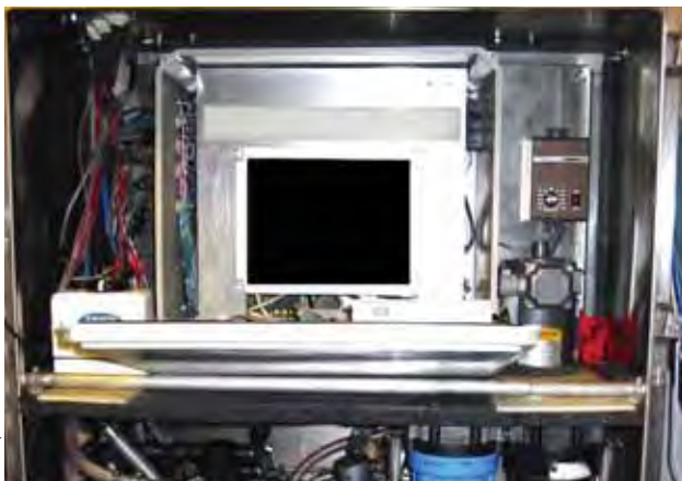
The primary instrument box on the Tustumena containing temperature, salinity, nitrate, chlorophyll and CDOM fluorescence, and optical transmittance sensors.
