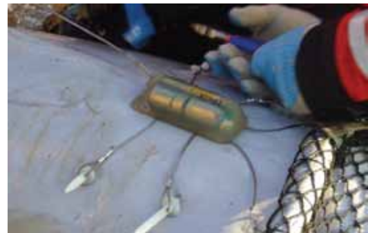
Satellite transmitter attached by cables to three nylon pins. Note that cables are not pulled tight so that they don't pull on the pins as the whale flexes and extends its dorsal surface as it swims.
