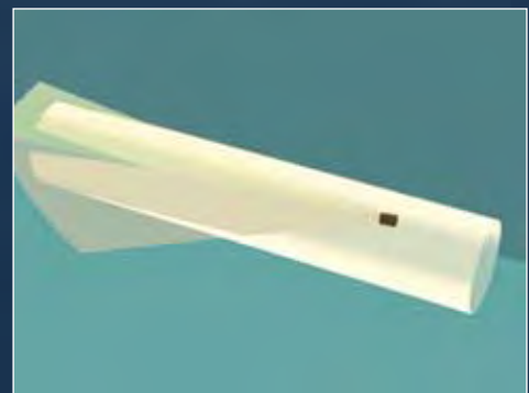
Orientation of the DIDSON sonar and the area that it imaged on the trawl net.
