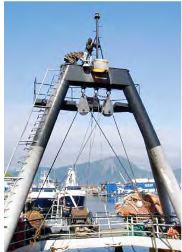
Technicians secure a downward-looking camera to trawler stern gantry.
