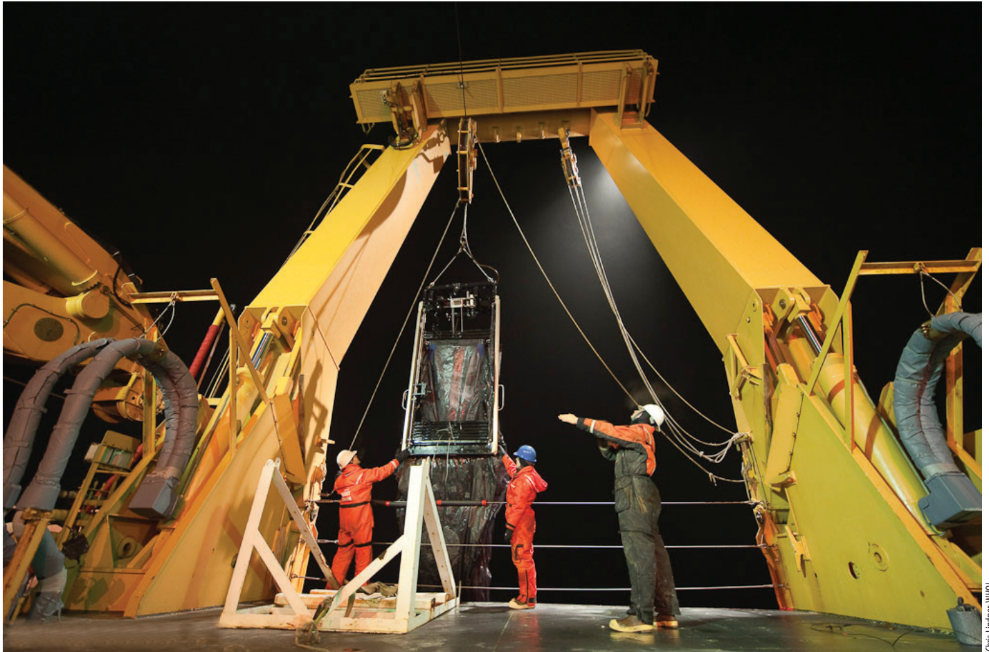
Nighttime deployment of the Multiple Opening/Closing Net and Environmental Sensing System (MOCNESS) off the stern of USCG Cutter Healy.
